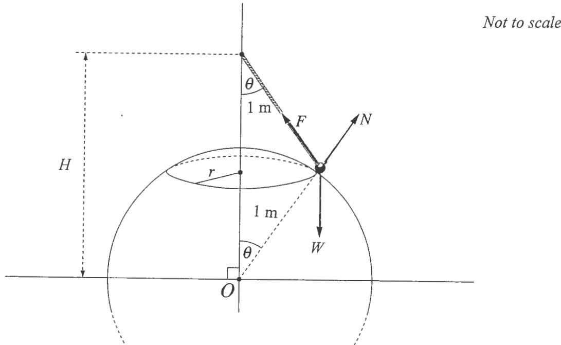
Three forces are acting on the bead: the tension force  $T$  of the string, the normal force  $N$  to the surface of the sphere and the gravitational force  $W$ . [All forces are in Newtons]. Take acceleration due to gravity as  $g \text{ m/s}^2$ .
