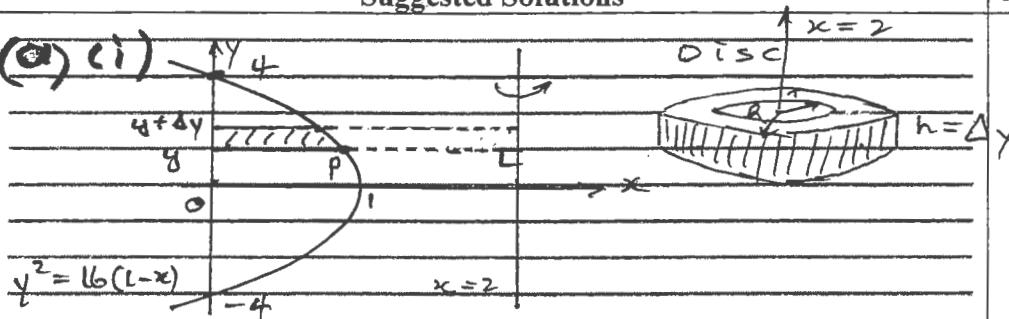
$$\text{CROSS-SECTIONAL AREA } A = \pi R^2 - \pi r^2 = \pi [R^2 - r^2] = \pi [R+r][R-r]$$
